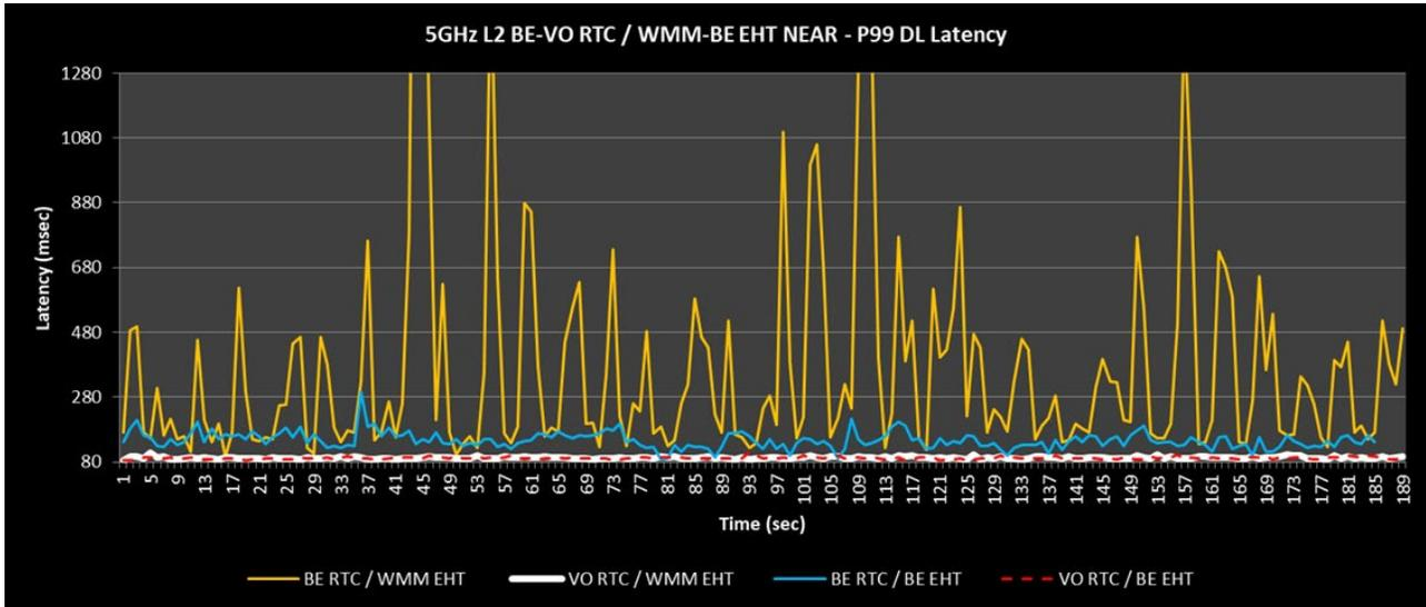
Figure 23. 5 GHz Level 2 Downlink Latency (Near Client)—Comparison of EHT on AC\_BE or WMM and RTC on AC\_BE or AC\_VO
