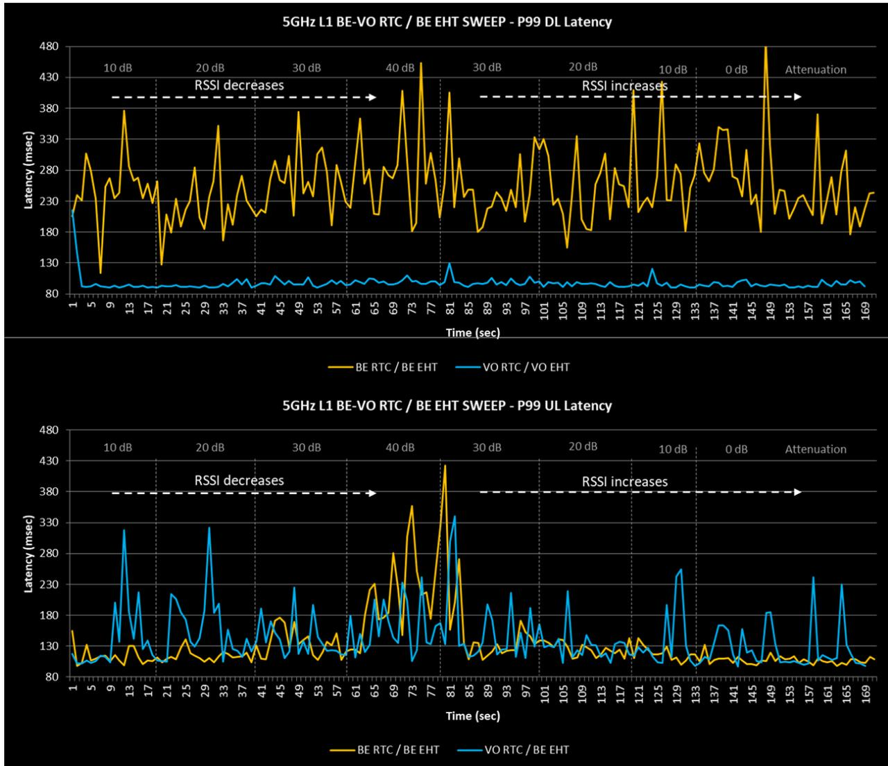
Figure 18. 5 GHz Level 1 P99 Latency (AC\_BE EHT)—Comparison of AC\_BE and AC\_VO for Downlink (top) and Uplink (bottom) When the Client RSSI (Attenuation) Changes (Sweep)
