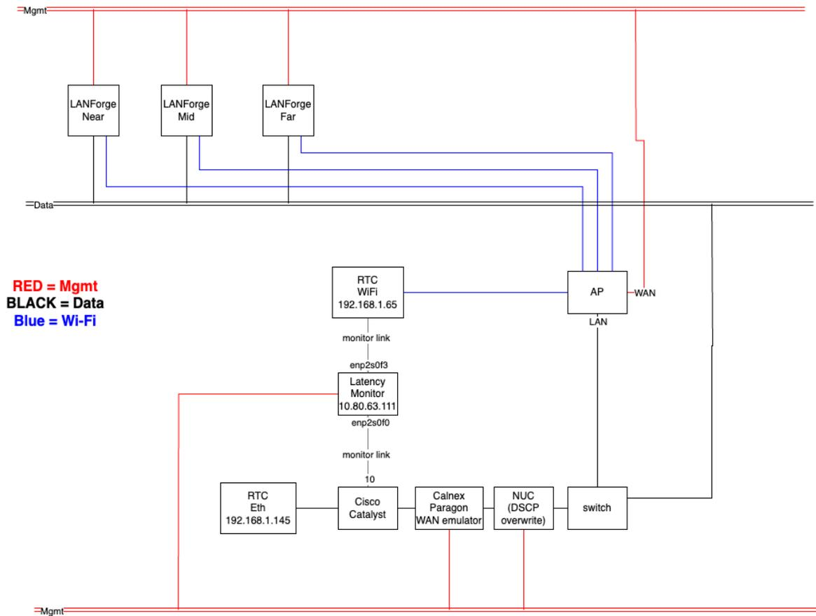
Figure 4. Network Topology of Wi-Fi QoE: Home in a Box
