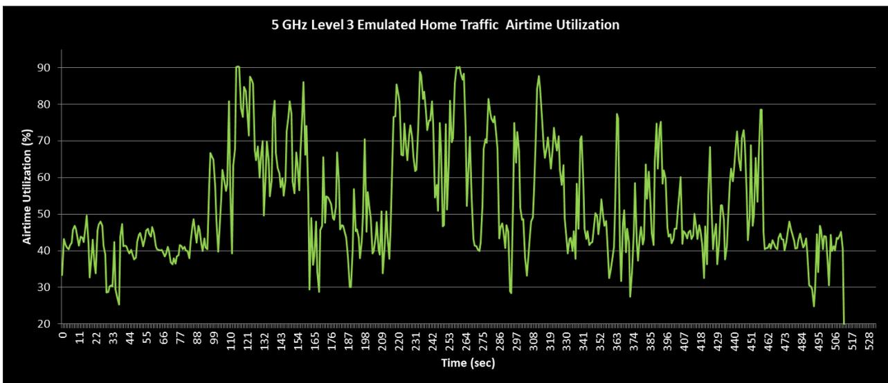
Figure 24. 5 GHz Level 3 Emulated Home Traffic Airtime Utilization (AC\_BE RTC, Mid Client)
