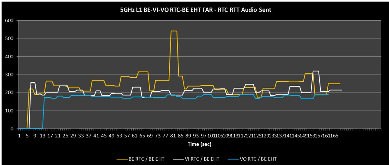
**Figure 17. 5 GHz Level 1 RTT Audio (AC\_BE EHT, Far Client)—Comparison of AC\_BE, AC\_VI, and AC\_VO**
