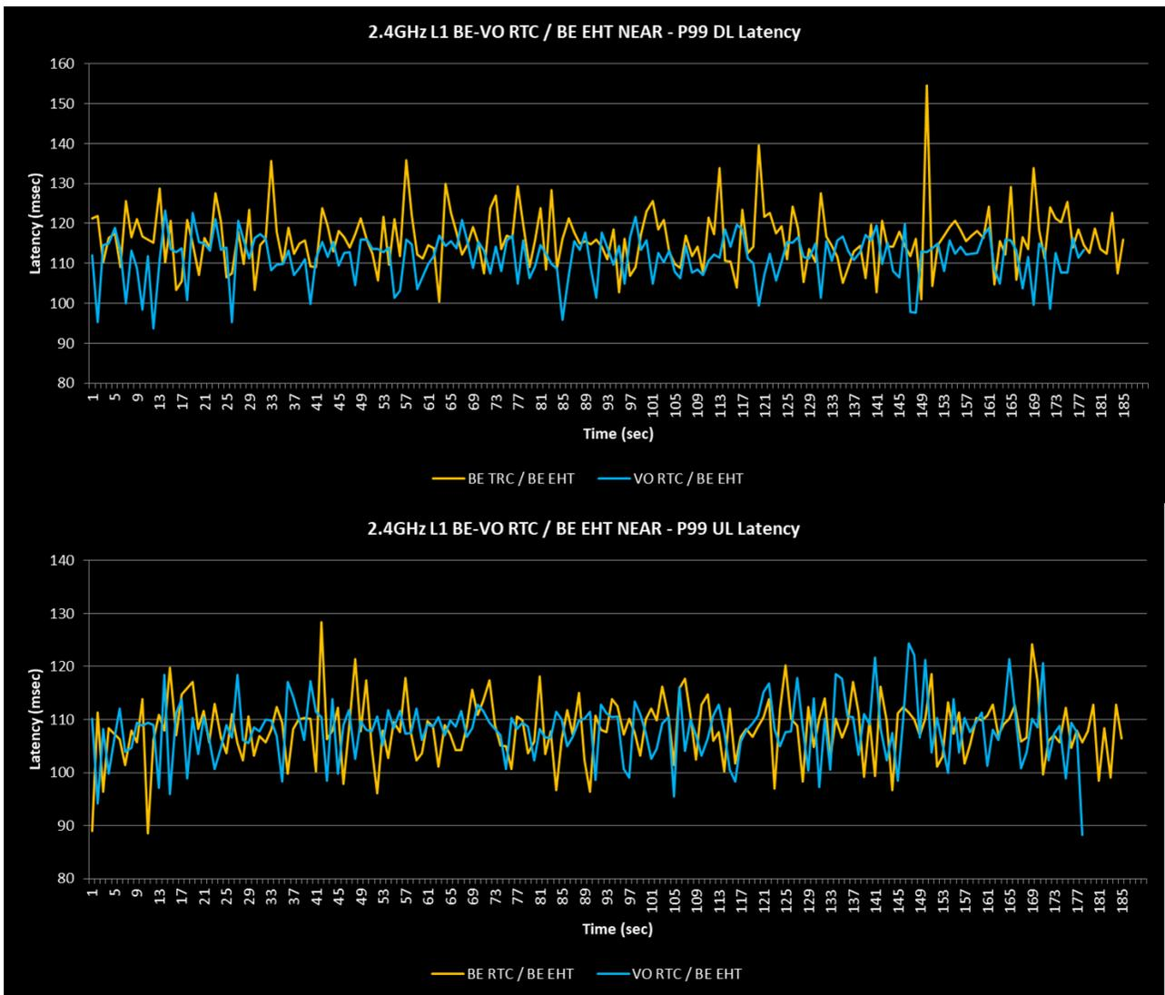
Figure 27. 2.4 GHz Level 1 P99 Latency (AC\_BE EHT, Near Client)— Comparison of AC\_BE and AC\_VO for Downlink (top) and Uplink (bottom)
