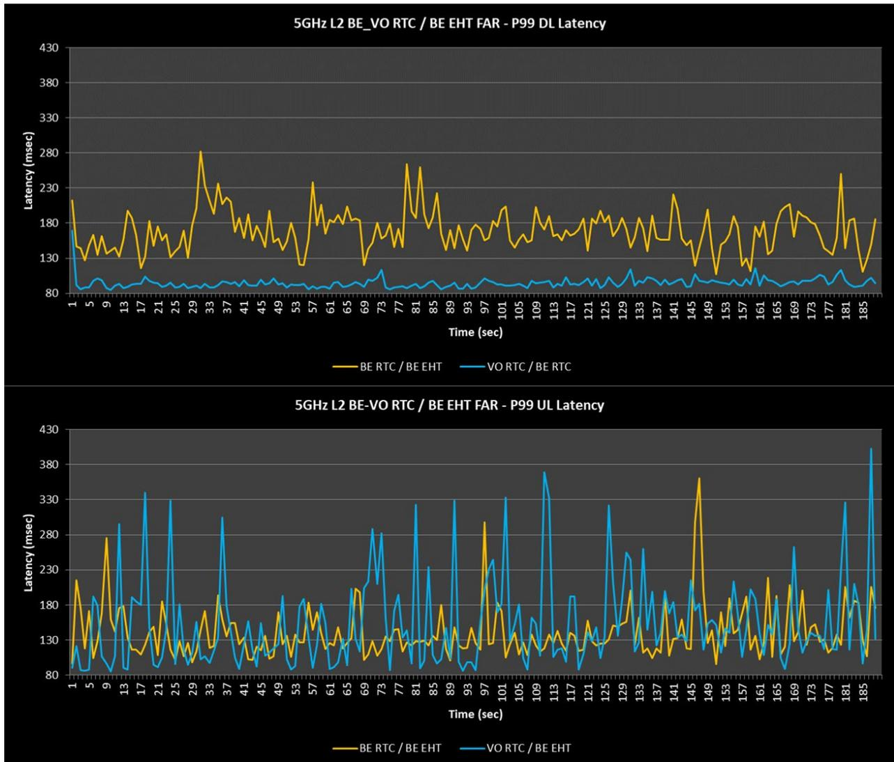
**Figure 22. 5 GHz Level 2 P99 Latency (AC\_BE EHT, Far Client)—
