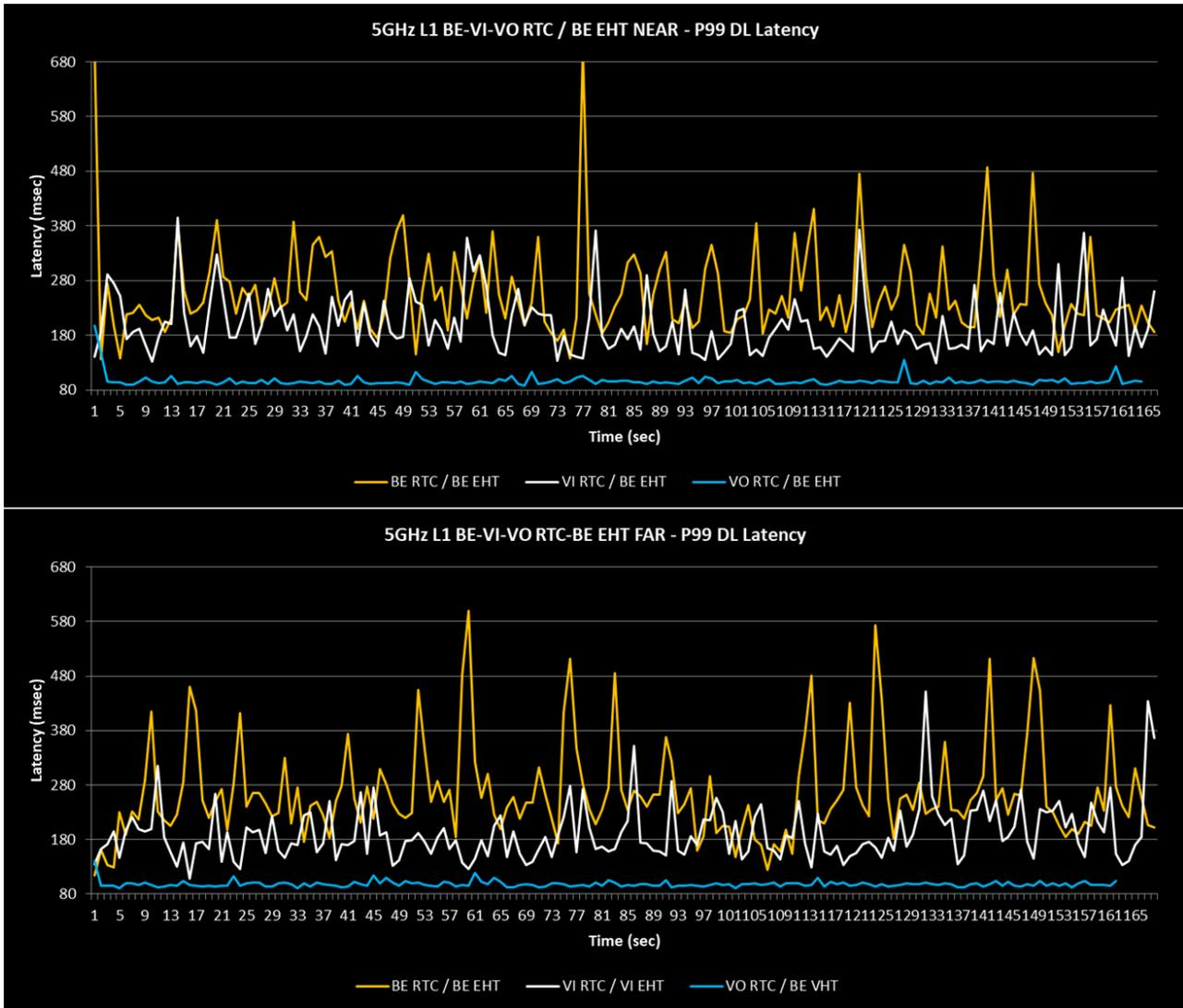
**Figure 15. 5 GHz Level 1 P99 Downlink Latency (AC\_BE EHT)— Comparison of AC\_BE, AC\_VI, and AC\_VO for a Near Client (top) and Far Client (bottom)**
