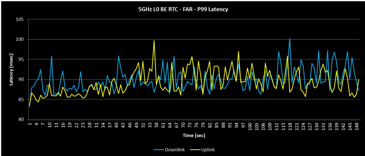
**Figure 13. 5 GHz Level 0 P99 Latency (AC\_BE, Far Client)—Comparison of Downlink and Uplink**
