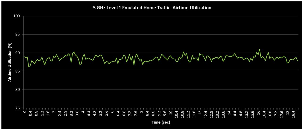
**Figure 14. 5 GHz Level 1 Emulated Home Traffic Airtime Utilization**
