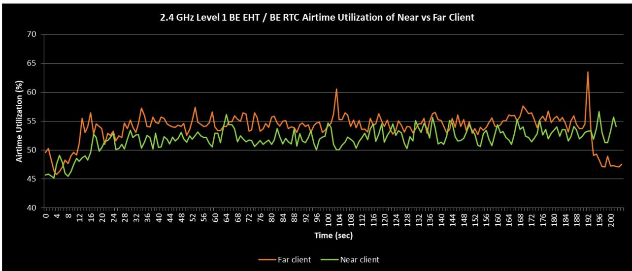
**Figure 26. 2.4 GHz Level 1 Airtime Utilization (AC\_BE EHT, AC\_BE RTC)—Comparison of a Near Client and a Far Client**
