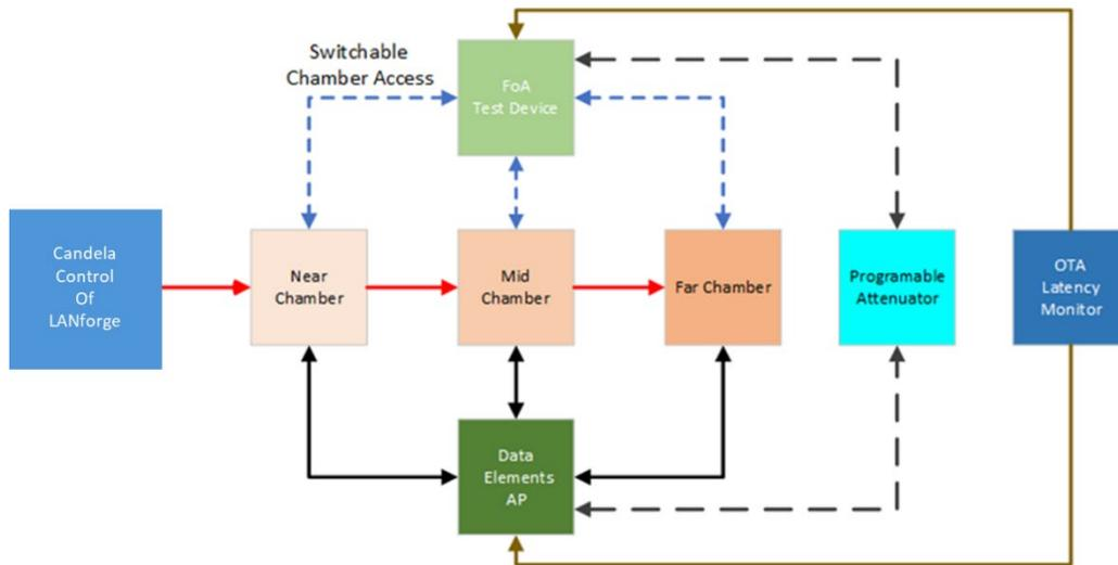
**Figure 3. Model Layout of Wi-Fi QoE: Home in a Box**
