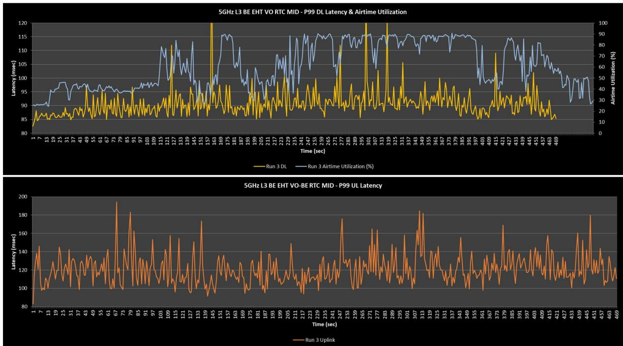
**Figure 25. 5 GHz Level 3 Downlink (top) and Uplink (bottom) Latency and Airtime Utilization (top) for Run 3 of AC\_VO RTC Test (AC\_BE EHT, Mid Client)**
