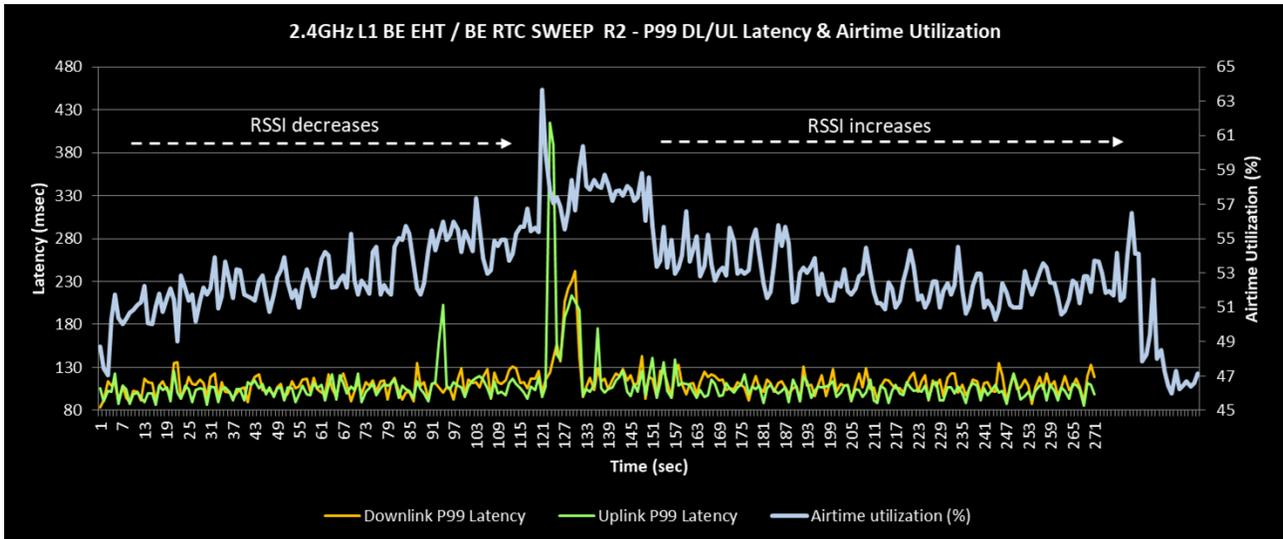
Figure 28. 2.4 GHz Level 1 P99 Latency (AC\_BE EHT, AC\_BE RTC)—Comparison of Downlink, Uplink, and Airtime Utilization When the Client RSSI (Attenuation) Changes (Sweep)
