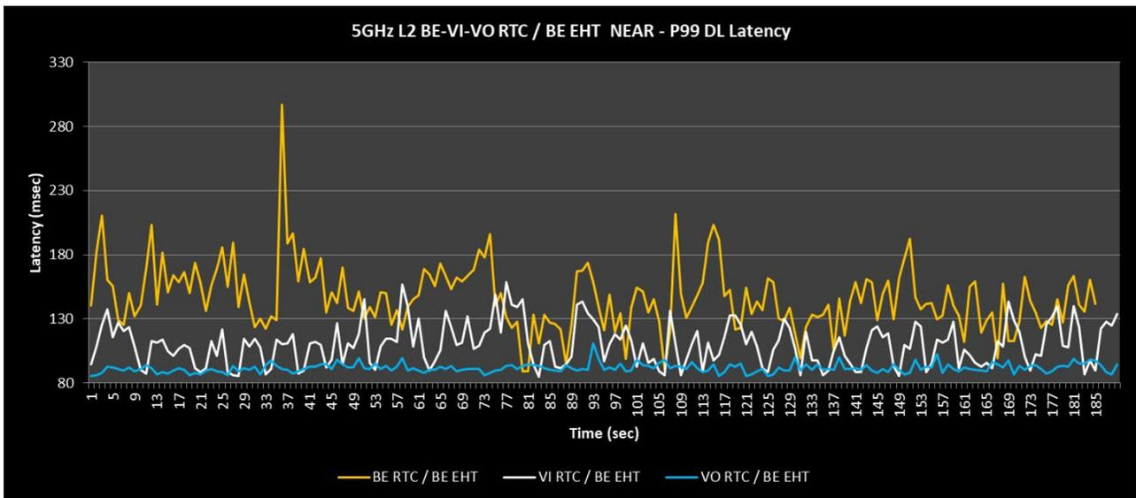
Figure 21. 5 GHz Level 2 P99 Downlink Latency (AC\_BE EHT, Near Client)— Comparison of AC\_BE, AC\_VI, and AC\_VO for RTC
