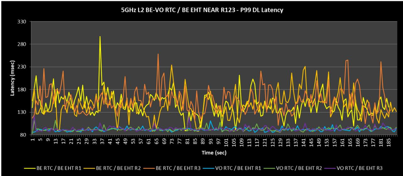
Figure 20. 5 GHz Level 2 P99 Downlink Latency (AC\_BE EHT, Near Client)— Comparison of AC\_BE RTC (3 Runs) and AC\_VO RTC (3 Runs)
