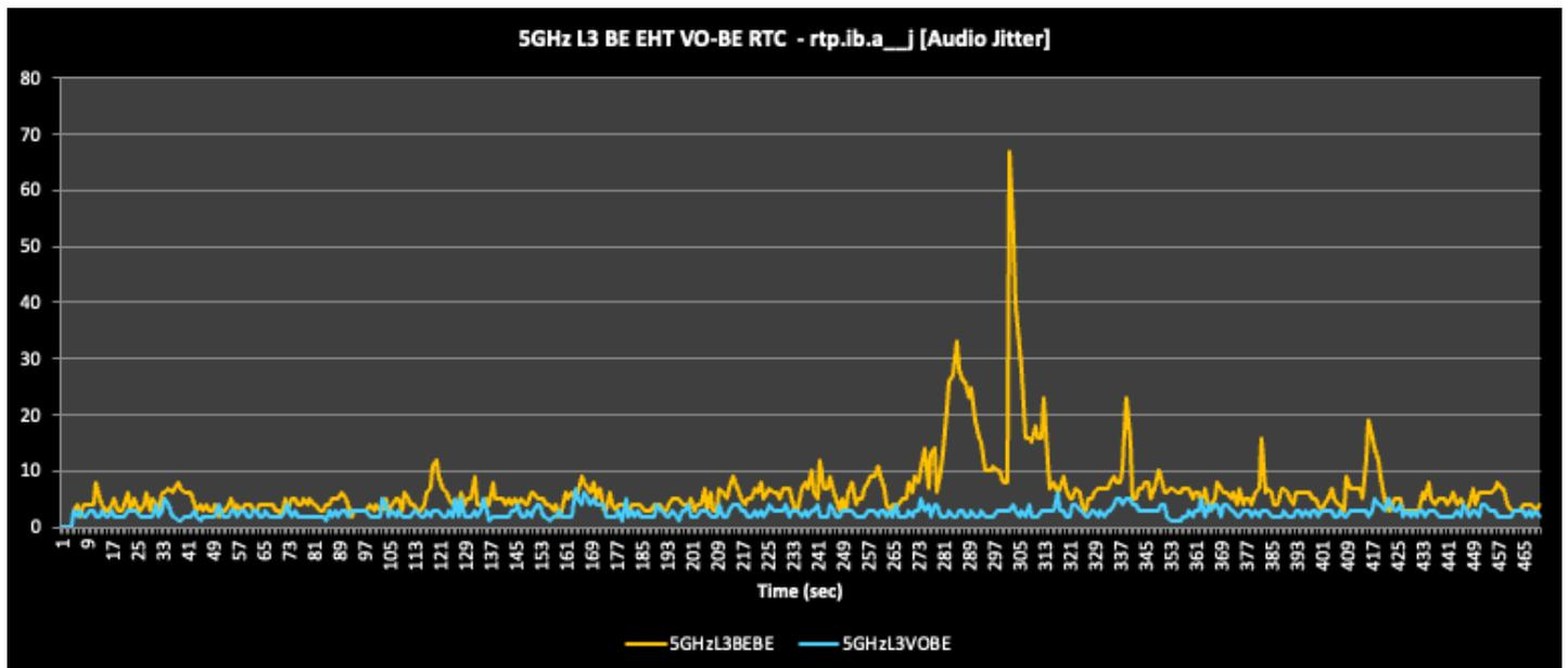
Figure 12. 5 GHz Level 3 Testing Results of Audio Performance
