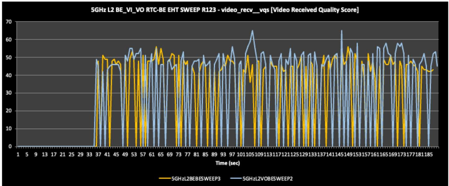
Figure 9. 5 GHz Level 2 Testing Results of Video Performance
