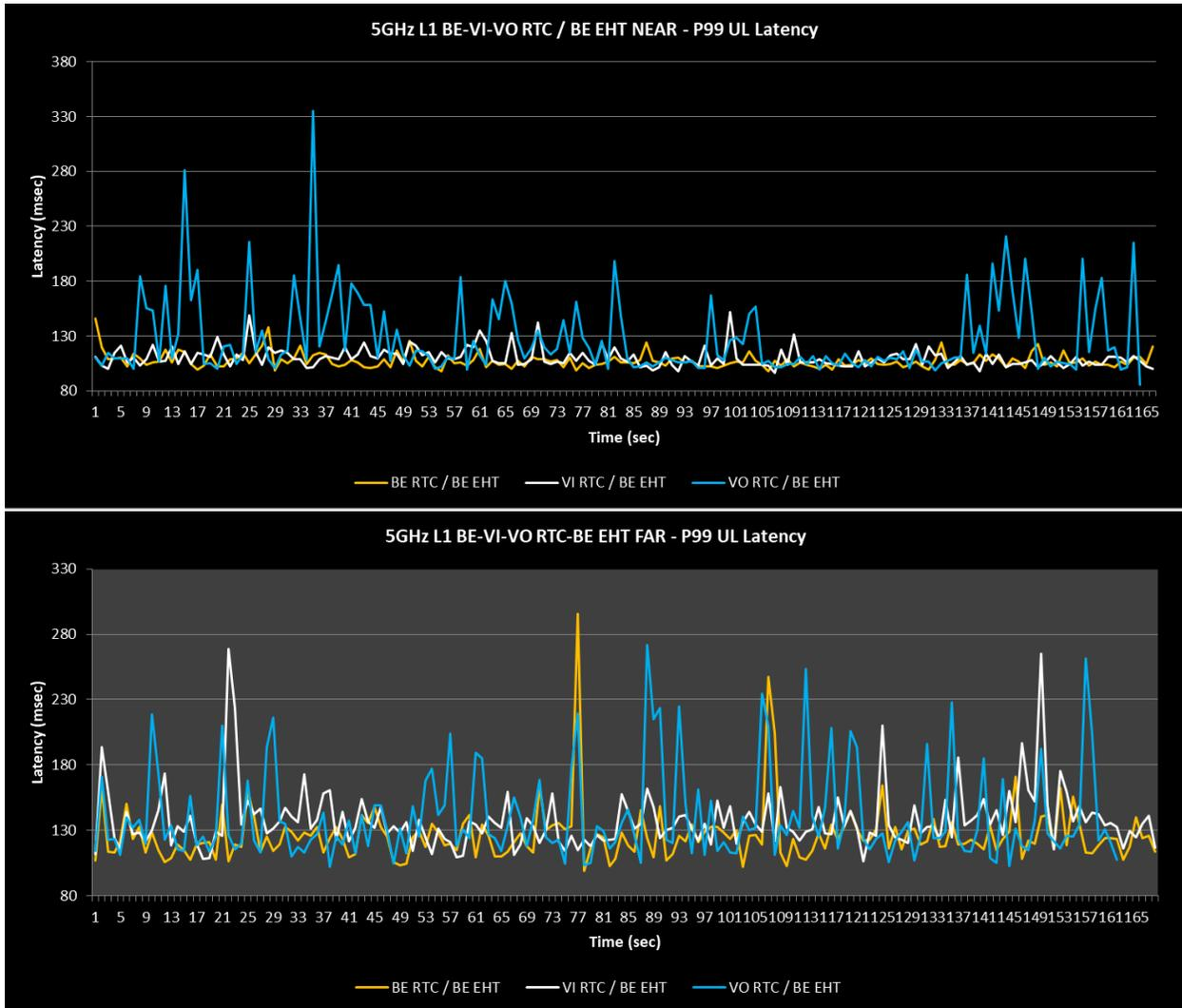
**Figure 16. 5 GHz Level 1 P99 Uplink Latency (AC\_BE EHT)— Comparison of AC\_BE, AC\_VI, and AC\_VO for a Near Client (top) and Far Client (bottom)**
