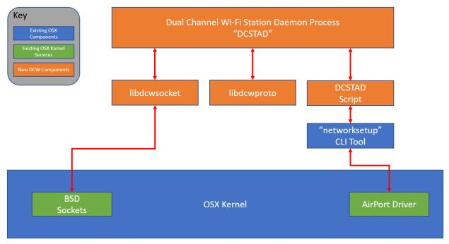
Figure 1 – OSX DCW Station S/W Architecture Overview
