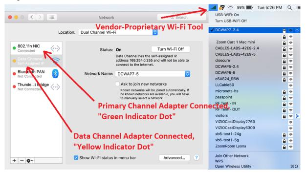
Figure 3 – System Preferences Network Pane Showing Bonded DCW
