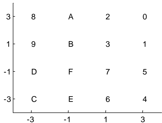
Figure A-4 - 16-QAM Constellation Mapping of \{y_0 y_1 y_2 y_3\}
