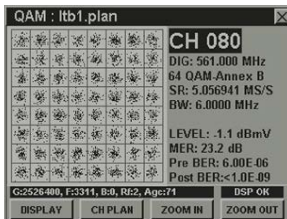
Figure I-26 - 64-QAM Signal With Poor (23.2 dB) MER
