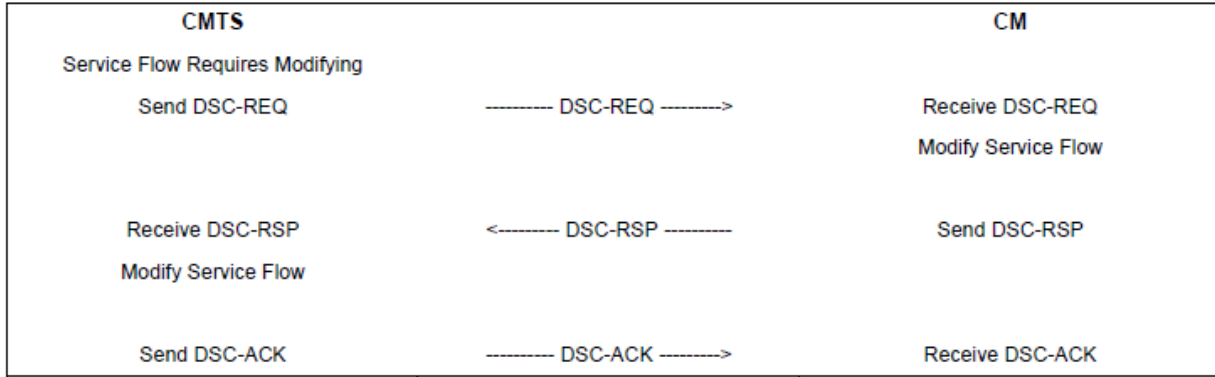
Figure 196 - CMTS-Initiated DSC Modifying a Service Flow
