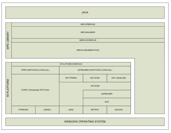
The RI Platform module is a mix and match of various external libraries, available under favorable licensing terms that we can incorporate into the CableLabs source code base as well as some CableLabs developed code. Its main purpose is to provide a multimedia framework that will allow the RI OCAP stack through the RI MPEOS implementation to use and excercise all of the multimedia features. That includes emulation of tuning, demultiplexing, decoding and displaying decoded content.
